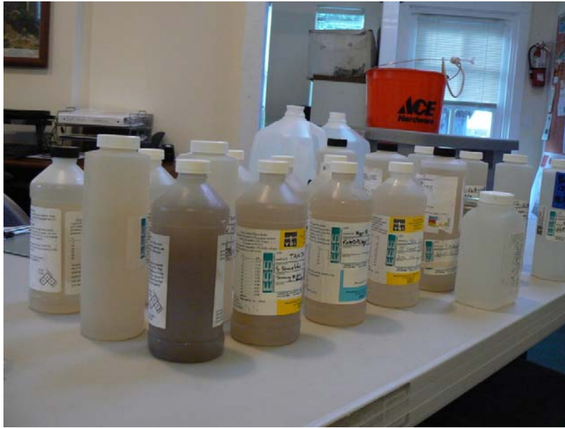
Turbidity samples collected at all stations during the 12/7 to 12/9 synoptic storm sampling
